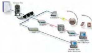
Typical topology of the UPS Network Management
