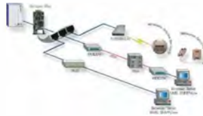
Typical topology of the UPS Network Management
