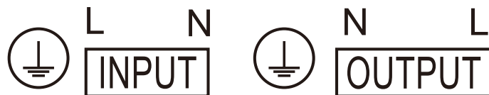
Fig 3:AC input/Output Connections
